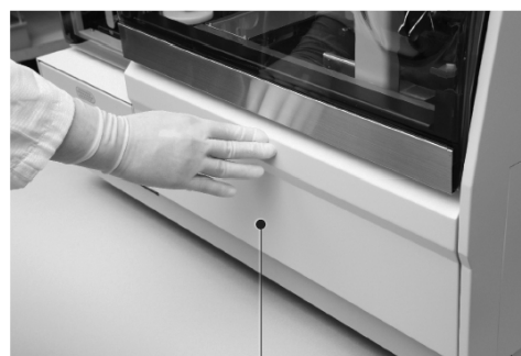
Loading station access door
