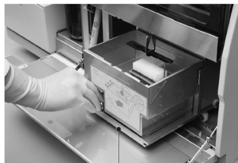
Loading station receiver
