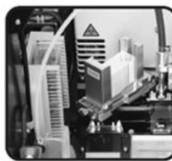
4: Delivery of slide into slide rack
