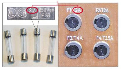
Four fuse holders, marked **F1** through **F4**, are located at the rear panel of the instrument, below the power supply sockets.
