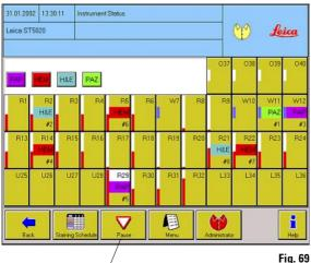
A staining process can be interrupted:
