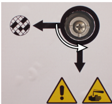
Figure 19. Vapor select valve in the external system position
