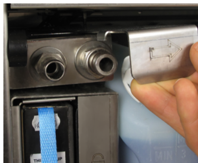
Figure 52. Remote fill/drain flap open with reagent line (left) and wax waste line (right)
